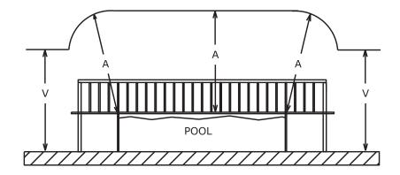
PERMANENTLY INSTALLED ABOVEGROUND SWIMMING POOL WITH DECK. CLEARANCE IS MAINTAINED FROM THE HIGHEST POINT OF THE INSTALLATION UPON WHICH PEOPLE CAN STAND,
