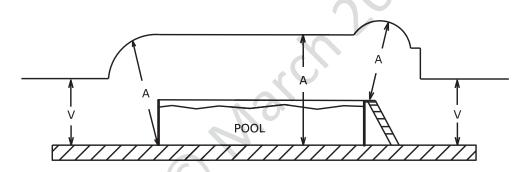
PERMANENTLY INSTALLED ABOVEGROUND SWIMMING POOL WITHOUT DECK. CLEARANCE IS MAINTAINED FROM THE HIGHEST POINT OF THE INSTALLATION UPON WHICH PEOPLE CAN STAND.
