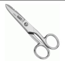
**Electrician's Scissors:** Scissors that have an upper blade that has notches for stripping 19- and 23-gauge wire. These are designed for telecom and electrical applications and heavyduty use. The serrated lower blade reduces slippage. These scissors are made with strong, tough tempered steel and have a nickel-plated finish that resists corrosion.
