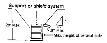
All excavations 20 feet or less in depth which have vertically sided lower portions that are supported or shielded have a maximum allowable slope of  $\frac{3}{4}$  H: 1V. The support or shield system must extend at least 18 inches above the top of the vertical side.
