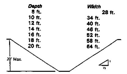
All simple slope excavations 20 feet or less in depth shall have a maximum allowable slope of 1 1/2H: 1V.
