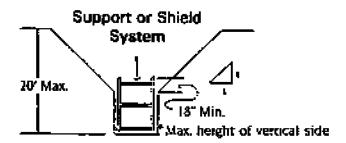
All excavations 20 feet or less in depth which have vertically sided lower portions shall be shielded or supported to a height at least 18 inches above the top of the vertical side. All such excavations shall have a maximum allowable slope of 1H: 1V.
