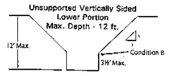
Excavations more than 8 feet but not more than 12 feet in depth which have unsupported vertically sided lower portions shall have a maximum allowable slope of 1H: 1V and a maximum vertical side of 3 ½ feet.
